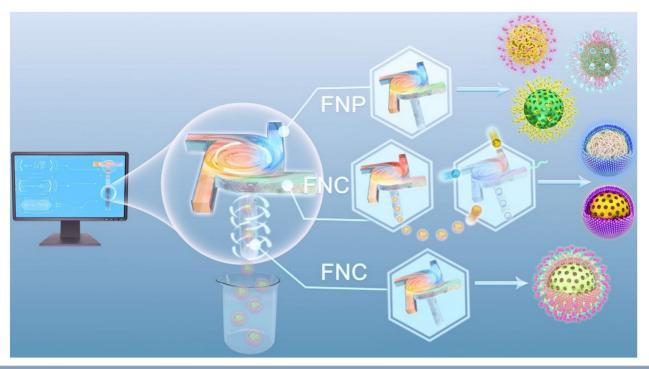
Flash-based self-assembly, from computational simulations to nanoparticle formulation. FNP produces polymeric and inorganic nanoparticles via solvent supersaturation. FNC produces nanoformulations using polyelectrolyte complexation driven by physical interactions such as electrostatic interactions, hydrogen bonding, and metal-coordination, and often involves the use of multiple devices in parallel for nanoparticle formation and surface modification.
