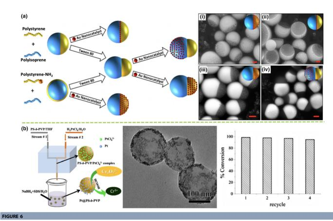
(a) Schematic and TEM images of FNP generation of Au-modified Janus and core–shell nano-hybrid. (Reprinted with permission from Ref. [119]. 2017, American Chemical Society.) (b) Schematic of FNP fabrication of Pt@PS-b-PVP nano-hybrid for Cr(VI) catalytic degradation to Cr(III); TEM image and recyclability test for reduction of Cr(VI) with four recycles. (Reprinted with permission from Ref. [106]. 2017, Springer Nature.)
